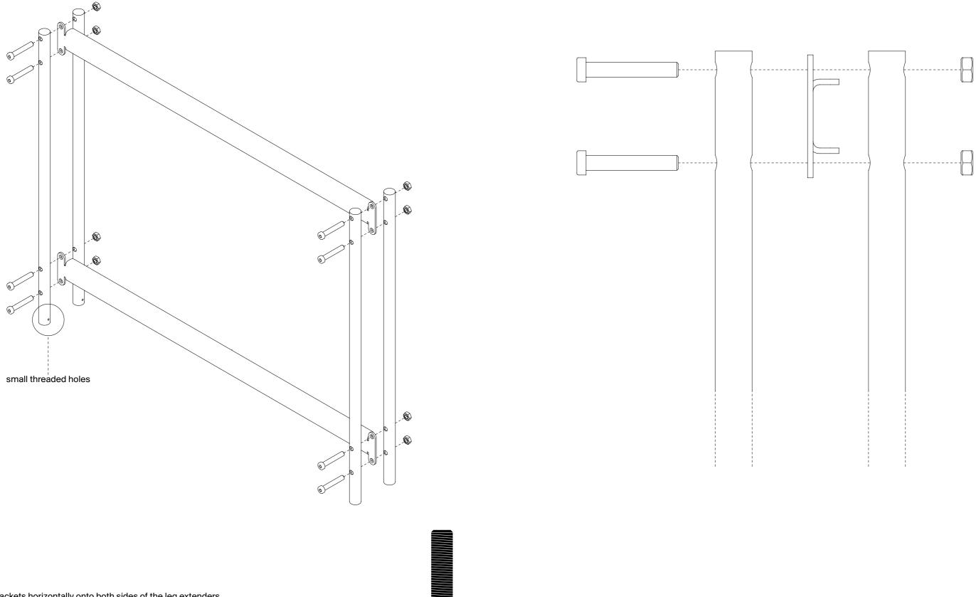
Mount the brackets horizontally onto both sides of the leg extenders as shown. Make sure to orient the small threaded holes inwards. Tighten all connections.
